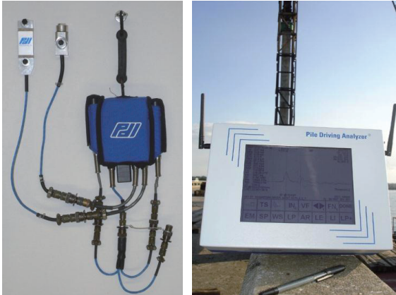
Figure 3. Strain and acceleration sensors, wireless data transmitter (left), Pile Driving Analyzer - Model PAX (right).
